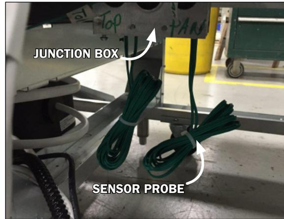
Fig. 9 Field-wired sensors
