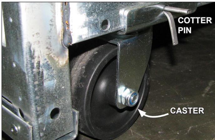
Fig. 1 Removing the casters is an easy process. Simply flatten and remove the cotter pins that are holding the casters in place. Then lift the case with a "J" bar and slide the caster assemblies out. The dismantled casters can now be discarded.
