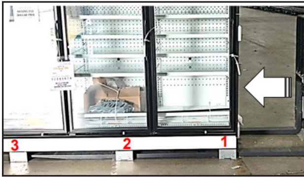
Fig. 5 Pallet blades extend past the second set of base feet
