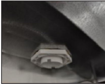
Fig. 6 If using a pallet jack, avoid damaging the drain hub (centered left-right on case)
