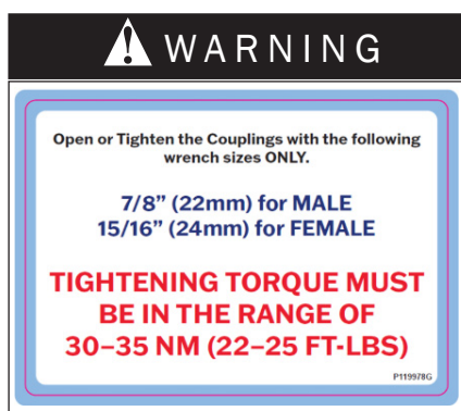
Fig. 26 Torque tightening requirements
