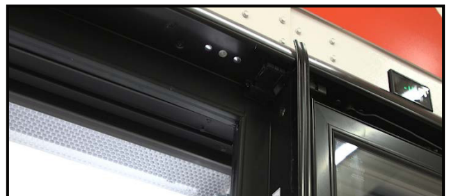
Fig. 75 Door frame trim installed
