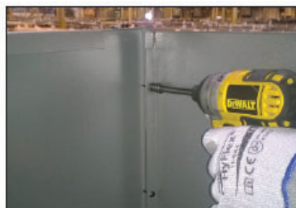
Fig. 8 Attach end panel to front fascia.
