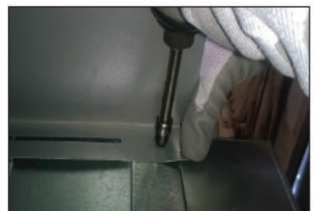
Fig. 9 Attach end panel to case body.
