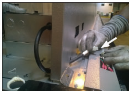
Fig. 5 Move electrical box forward and connect heater wire.
