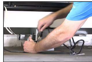
Fig. 51 Plug pump into pump receptacle
