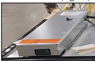
Fig. 92 Switch location on junction box
