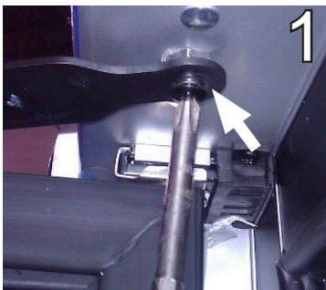
Fig. 67 Disconnect hold-open assembly
