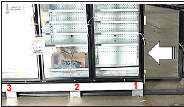
Fig. 22b Pallet blades extend past the second set of base feet
