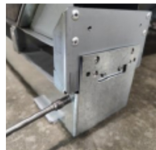
Fig. 40 Fasten front plates to side fastening holes
