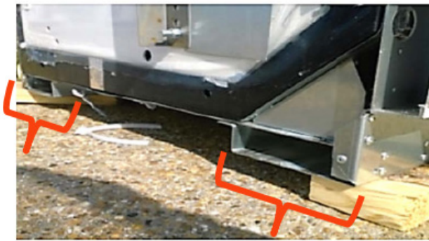
Fig. 22a Base feet lifting points
