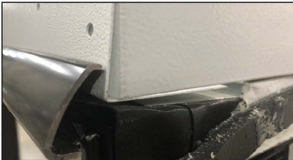
Fig. 79 Align the front fascia to the curved flange of door
