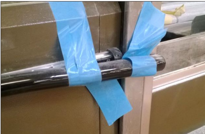
Fig. 11 Leave 6 inches of extra bumper
