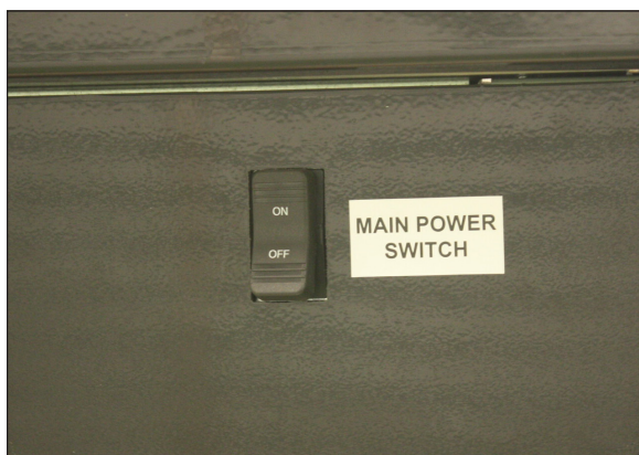
Fig. 9 Lower panel power switch
