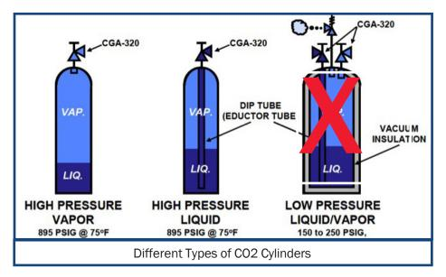
Note: Low-Pressure Liquid/Vapor cylinders are not recommended for use with booster systems due to their lower pressure ratings.
