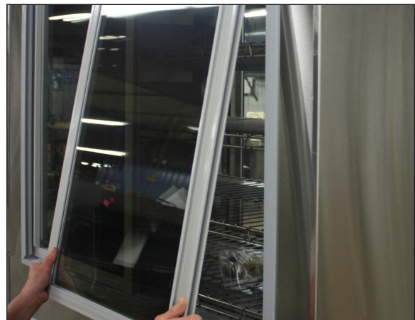
Fig. 11 Rear load door removal
