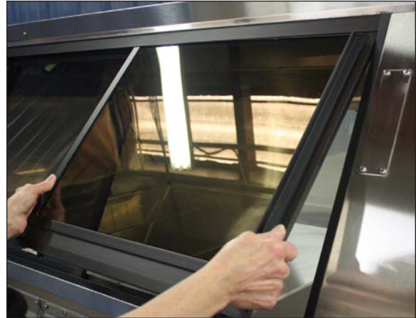
Fig. 5 Rear load door removal
