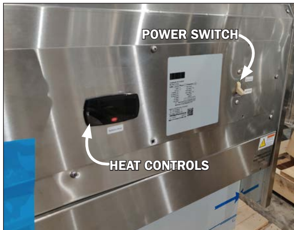
Fig. 4 Digital heat controls & hinged cornice access panel
