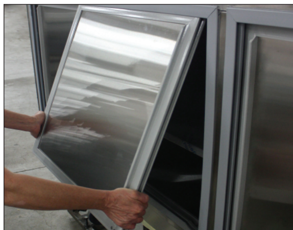
Fig. 17 Front lower door removal
