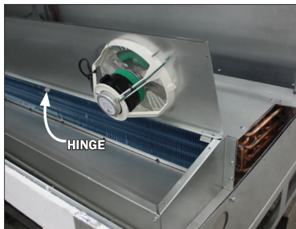
Fig. 15 Pressure plate and hinges (underside)
