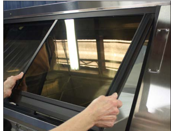
Fig. 5 Rear load door removal
