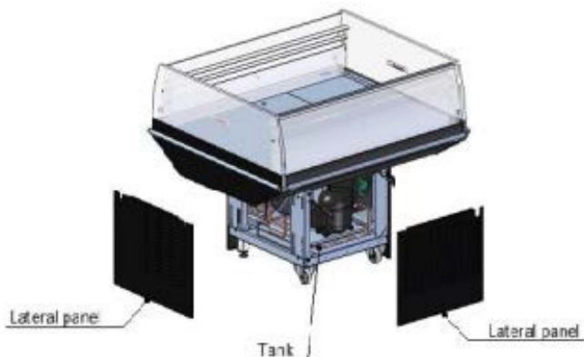
Fig. 15 Removing condensating unit panels
