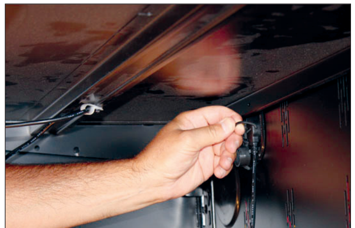
Fig. 11 Unplug the LED luminaire
