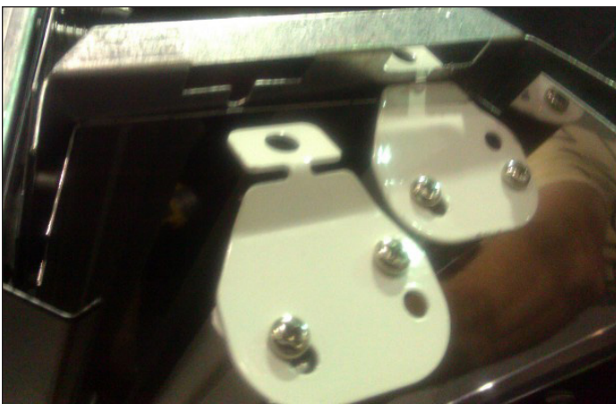
Fig. 14 Slide the other end to the opening in the sheet metal and disengage
