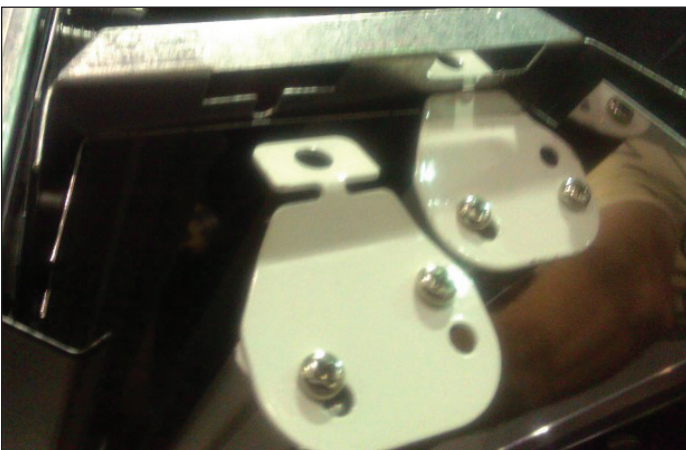
Fig. 17 Slide the other end to the opening in the sheet metal and disengage
