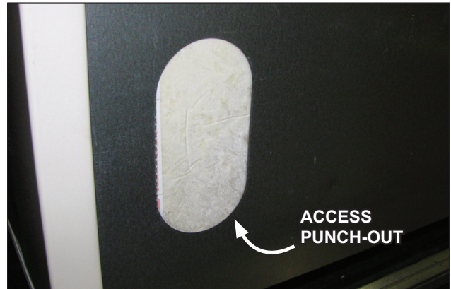
Fig. 11 Penetrate foam as needed to access piping
