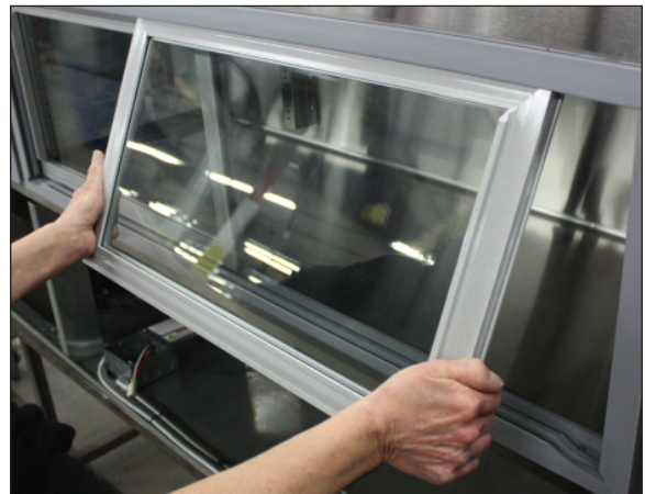
Fig. 18 Rear lower door removal
