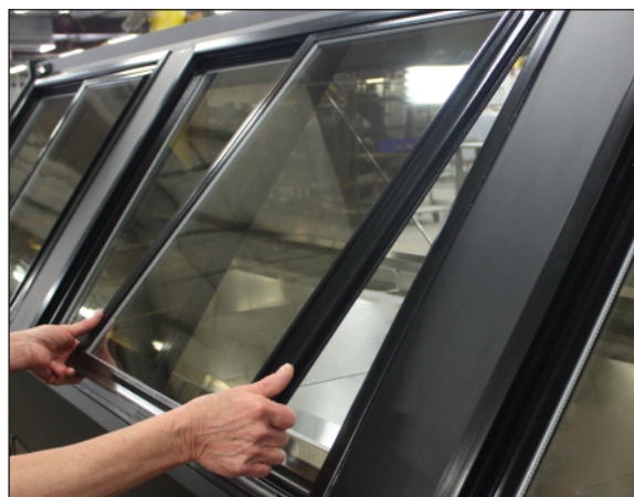
Fig. 19 Rear load door removal
