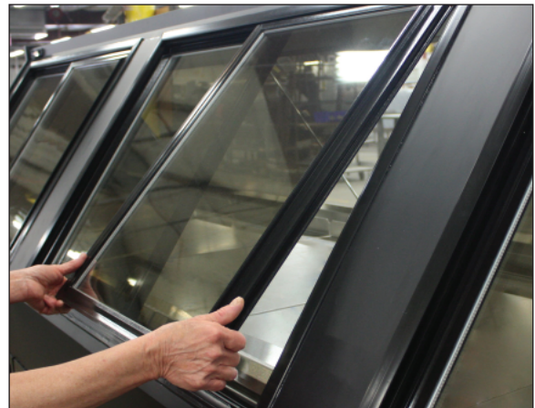
Fig. 17 Rear load door removal
