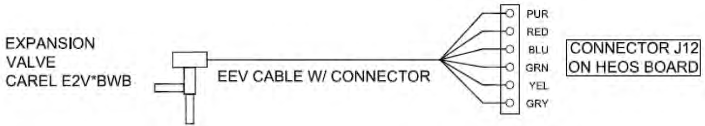
Fig. B-6 EEV Cable Connection to HEOS Control Board Location
