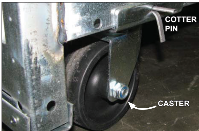
Fig. 1 Removing the casters is an easy process. Simply flatten and remove the cotter pins that are holding the casters in place. Then lift the case with a "J" bar and slide the caster assemblies out. The dismantled casters can now be discarded.
