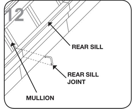
Install the rear sill joint that is provided. The bottom portion of the joint should be slid on the the rear sill first, then the top lip fits between the rear sill and the mullion. Secure the joint underneath the rear sill with the screws provided.
