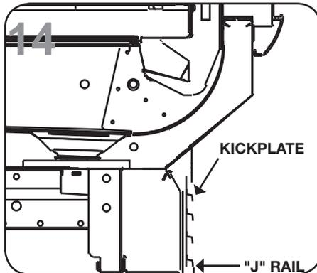
Slide the kickplate up and behind the lower front panel bracket, then down on the "J" rail.
