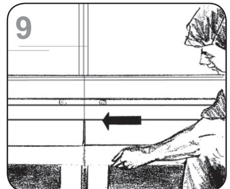
9 Close the joints of the front panel. The panel is slotted on the bottom to allow left-or-right adjustment as required.
