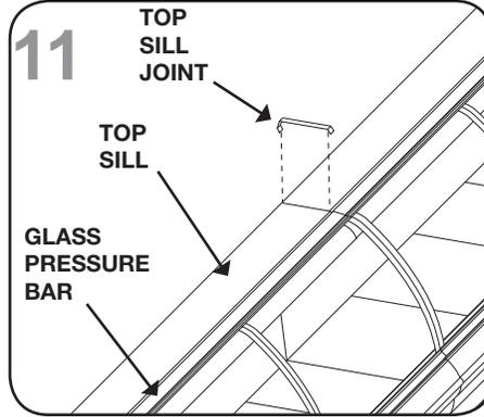
Install the top sill joint that is provided. The front lip of the joint fits into the crevice between the top sill and the glass pressure bar. The rear lip is attached to the back of the case with the screws provided.
