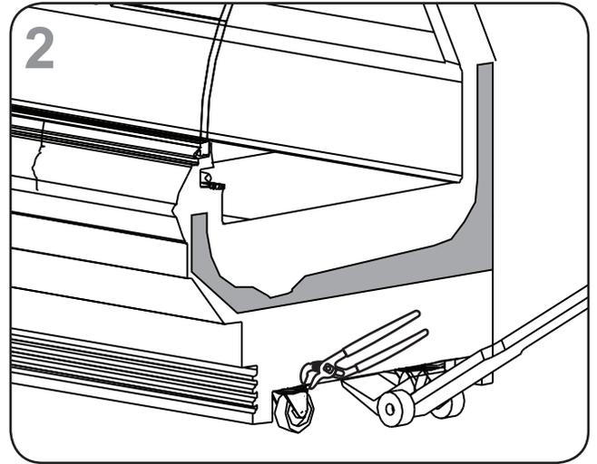
**IMPORTANT:** If skid boards are required for unloading cases, casters should be removed prior to sliding cases down the skid (see Diagram 3). When unloading is complete, re-install the casters.
