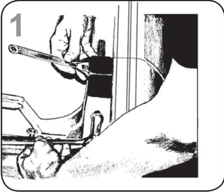
1 Tighten all joint bolts tightly, but do not over tighten.
