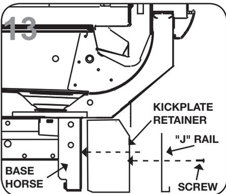
Attach the kickplate retainers to the basehorse, then mount the "J" rails to the kickplate retainers with the screws provided.
