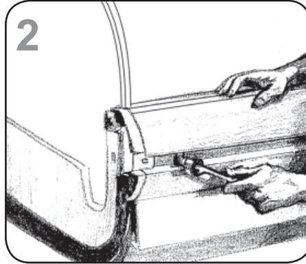
2 Adjust the polymer master bumper joints, if required. Loosen the bumper screws first.
