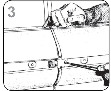
3 Slide the bumper joint to the center of the joint between the two cases. Use screw driver in hole provided.
