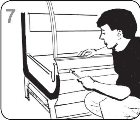
Loosen screws on the master bumper. Move bumper joint to a position for sliding between adjoining case bumper.
