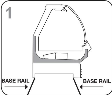
Using chalk lines, mark the floor where cases are to be located for the entire lineup. Snap lines where the base rails are positioned — not the front or back edges of the cases.
