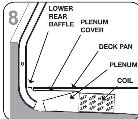
8 Install the plenum covers under deck pans, between the lower rear baffle and the fan plenum.
