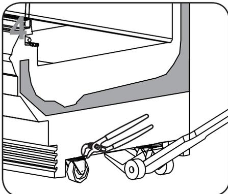
Roll the first case into position. Raise case from the end under cross support using "J" bar. Remove cotter pins and casters. Level the case on shims.
