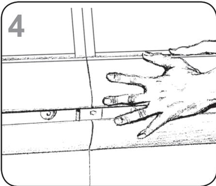
4 Slide the master bumper left or right to close seam as required. Bumper joint neatly finishes any gap that may remain.
