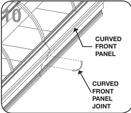
Install the curved front panel joint (if applicable) that is provided. Wide joints (1") are for case-to-case joining and narrow joints (1/2") are for cases with ends.
