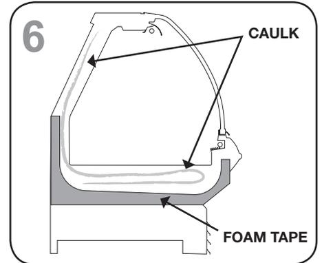
Remove anything from the case that may interfere with case joining. Apply the foam tape that is shipped loose in the case to the end breakers on each side of the case. Run a bead of sealant around the entire end before pushing cases tightly together.
