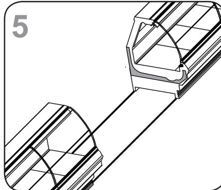
Roll case approximately 2' from adjoining case, then remove casters on that end. With the opposite end's casters still in place, push the cases together. Remove remaining casters.
