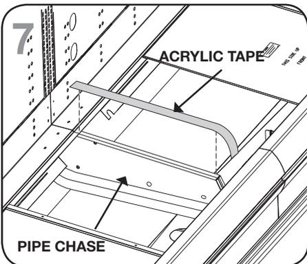
7 Apply the provided acrylic tape over the pipe chase seam. The tape acts as a watershed, preventing water from settling in case joint.
