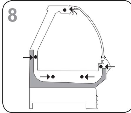
Push cases tightly together. Bolt cases together through the five holes provided in the "C" frame and pipe chase as shown in illustration. Tighten until all margins are equal; do not over tighten.
