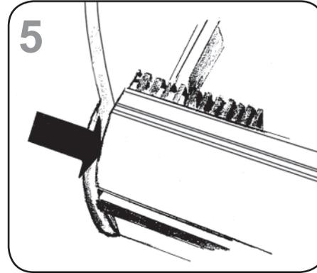
5 Close the seam where the bumper joins the case end. The bumper joint closes the seam that may develop if the master bumper is moved away from end in order to close the case-to-case joint seam.
