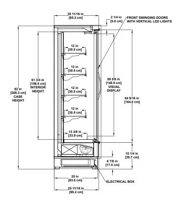
Please consult Hillphoenix Engineering Reference Manual for dimensions, plan views and technical specifications. Specifications subject to change without notice. Designed for optimal performance in store environments where temperature and humidity do not exceed  $75^\circ$  F and 55% R.H. Certified to UL 471 and 4NSI/NSF Standard 7.
