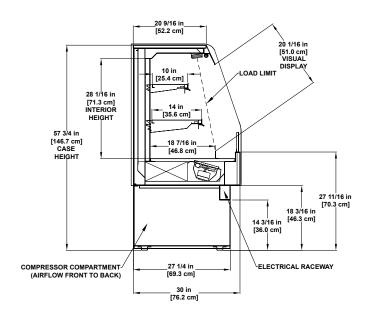
Please consult Hillphoenix Engineering Reference Manual for dimensions, plan views and technical specifications. Specifications subject to change without notice. Designed for optimal performance in store environments where temperature and humidity do not exceed 75° F and 55% R.H. Certified to UL 471 and ANSI/NSF Standard 7.
