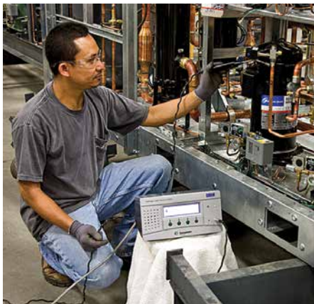
Systems are leak-tested during production with a safe, green-labeled gas.
