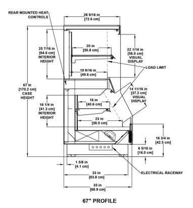
Please consult Hillphoenix Engineering Reference Manual for dimensions, plan views and technical specifications. Specifications subject to change without notice. Designed for optimal performance in store environments where temperature and humidity do not exceed 75° F and 55% R.H. Certified to UL 471 and ANSI/NSF Standard 4 and 7.
