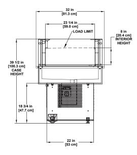
Please consult Hillphoenix Engineering Reference Manual for dimensions, plan views and technical specifications. Specifications subject to change without notice. Designed for optimal performance in store environments where temperature and humidity do not exceed 75° F and 55% R.H. Certified to UL 471 and ANSI/NSF Standard 7.
