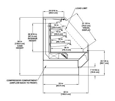
Please consult Hillphoenix Engineering Reference Manual for dimensions, plan views and technical specifications. Specifications subject to change without notice. Designed for optimal performance in store environments where temperature and humidity do not exceed 80° F and 55% R.H. Certified to UL 471 and ANSI/NSF Standard 7.
