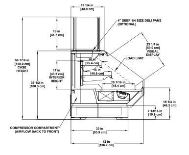
Please consult Hillphoenix Engineering Reference Manual for dimensions, plan views and technical specifications. Specifications subject to change without notice. Designed for optimal performance in store environments where temperature and humidity do not exceed  $80^\circ$  F and 55% R.H. Certified to UL 471 and ANSI/NSF Standard 7.
