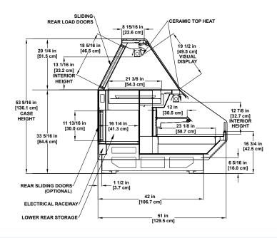
Please consult Hillphoenix Engineering Reference Manual for dimensions, plan views and technical specifications. Specifications subject to change without notice. Designed for optimal performance in store environments where temperature and humidity do not exceed 75° F and 55% R.H. Certified to UL 471 and ANSI/NSF Standard 4.
