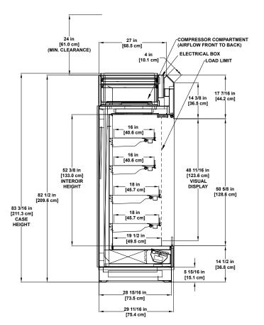
Please consult Hillphoenix Engineering Reference Manual for dimensions, plan views and technical specifications. Specifications subject to change without notice. Designed for optimal performance in store environments where temperature and humidity do not exceed 75° F and 55% R.H. Certified to UL 471 and ANSI/NSF Standard 7.
