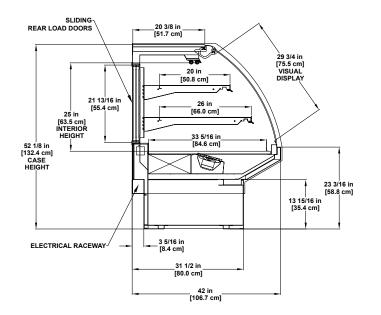
Please consult Hillphoenix Engineering Reference Manual for dimensions, plan views and technical specifications. Specifications subject to change without notice. Designed for optimal performance in store environments where temperature and humidity do not exceed 75° F and 55% R.H. Certified to UL 471 and ANSI/NSF Standard 7.
