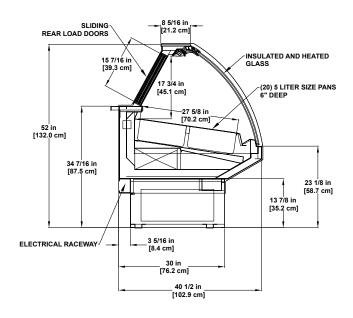
Please consult Hillphoenix Engineering Reference Manual for dimensions, plan views and technical specifications. Specifications subject to change without notice. Designed for optimal performance in store environments where temperature and humidity do not exceed 75° F and 55% R.H. Certified to UL 471 and ANSI/NSF Standard 7.
