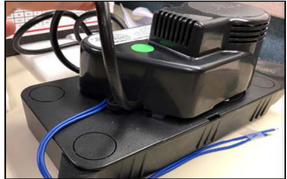
Pump with wiring and tubing
