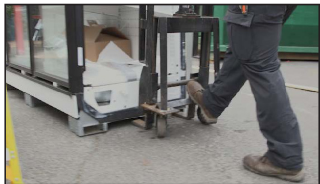
If using a pallet jack, avoid damaging the drain hub (centered left-right on case).
