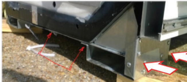
Case supported by wood blocks with lift points shown
